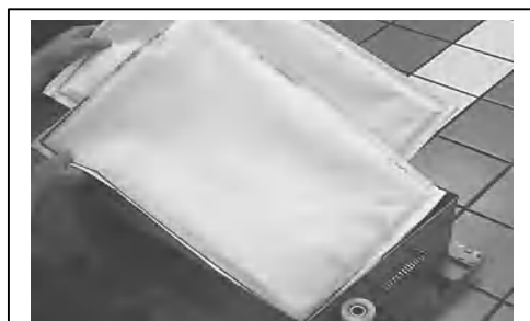
Installing new filter paper.
