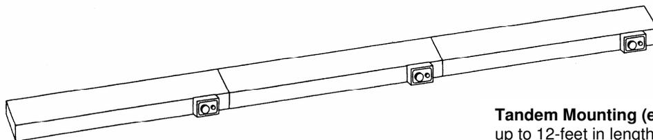
**Tandem Mounting (end-to-end)** – Overhead warming up to 12-feet in length.
