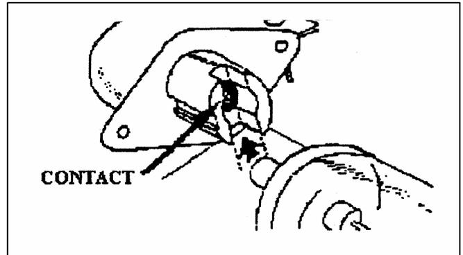
2. Place the left tip of the tube under the white socket (receptacle of the terminal). Raise the tube into the slot and apply enough inward pressure to compress the terminal slightly.
