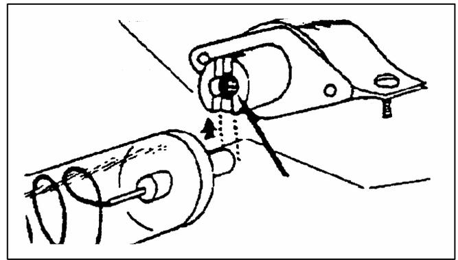
4. Raise the tube into direct alignment with the center of the right terminal. Release grip slowly allowing the compressed left socket (terminal) to lock tube into position.
