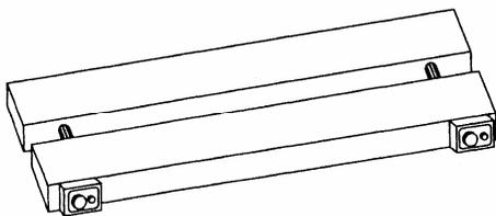
**Dual Mounting (side-to-side)** – Overhead warming in any width. 4-inch spacing standard.
