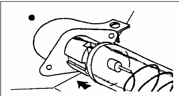
3. While keeping the tube compressed into the left terminal of the socket, position the right end of the tube directly beneath the right socket.
