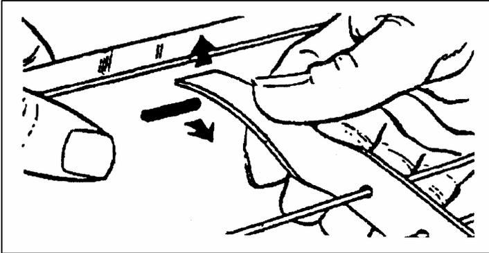
1. Remove the tube guard by pushing against the face of the warmer with left thumb and “bowing” the cross brace upward with your right hand. Pull the brace free. Remove the lengthwise brace.
