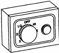
**Infinitely Adjustable Heat Controls** – “Dial-in” the perfect temperature for any food. Includes pilot light.
